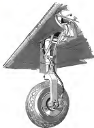
Acad landing gear used on Globe Swift reflects into well just ahead of main gear. Designed for load factor of 4.23 on 1,750-lb. plane, this gear accommodates standard 600 x 6 tires mounted on split-type wheel drums.
